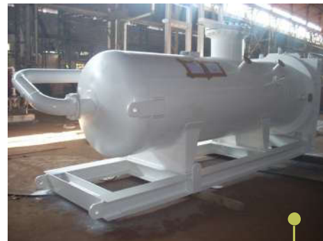
Vent Gas / Closed Drain Vessel
