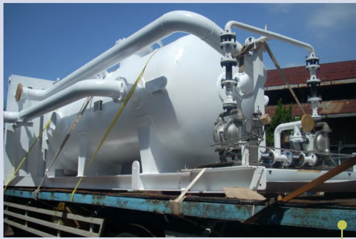
Flare Gas Scrubber
