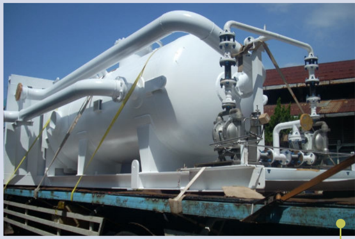
Flare Gas Scrubber
