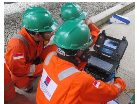
Inspection inside Tube and Hole by Borescope
