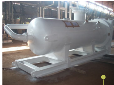
Vent Gas / Closed Drain Vessel
